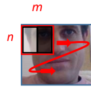
Figure 10 – Balayage de type raster
